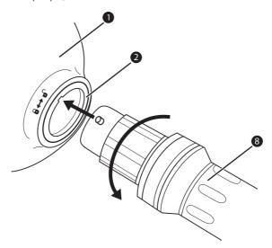
◆ Afterwards, insert the hose fitting on the other side of the air hose 8 firmly into the connection-support of the air-bubble mat ②.
